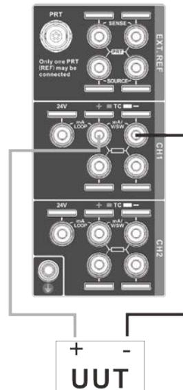
Figure 5 Connection way of Electric Current(mA) Measurement
