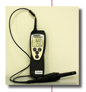
The **Model 625** humidity/temperature hand-held hygrometer can display any of the following: RH and temperature, or dew point and temperature, or wet bulb and temperature. The unit includes the 625 hand held hygrometer, an integral humidity probe head, a handle and cable, a 9V battery, a travel case and a NIST traceable calibration certificate.
